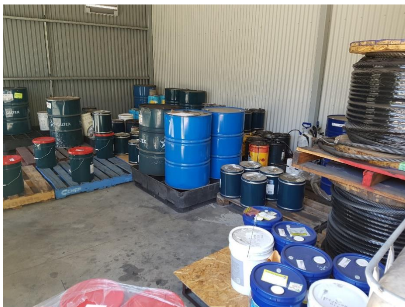
Plate 1A: Inconsistent storage of oil and lubricant drums (some on spill pallets, some not) at Workshop store (Before Photo)
