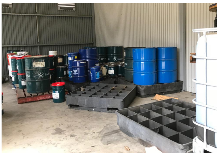
Plate 2B: Drums of grease are stored on wooden pallets, oil and lubricant drums stored on bunded pallets at Workshop store (After Photo)
