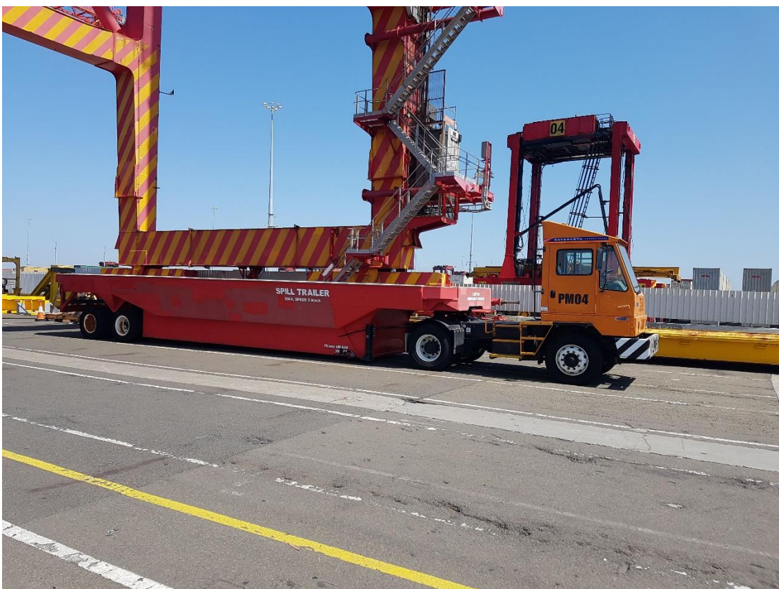
Plate 9: Purpose built spill trailer for moving leaking shipping containers
