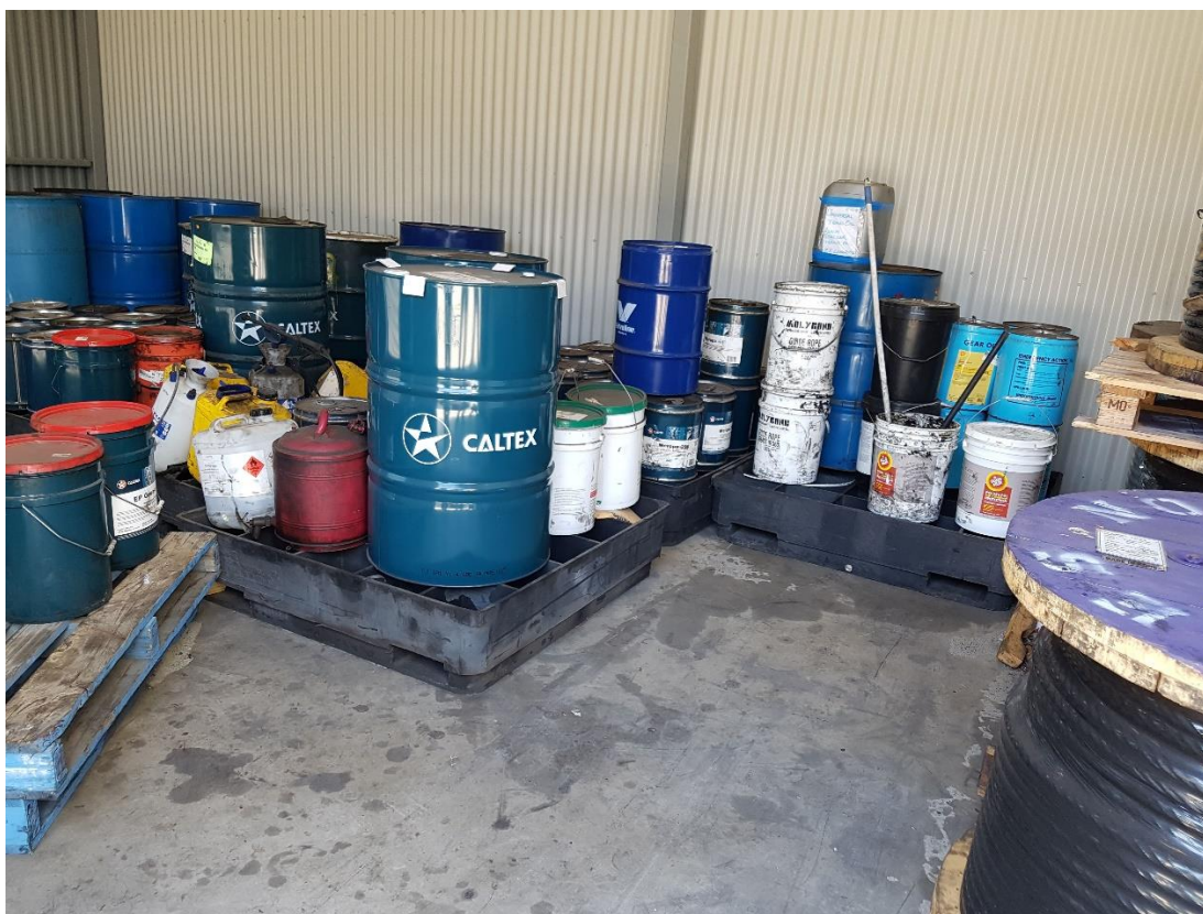
Plate 1: Appropriate storage of liquid oil and lubricant drums on spill pallets at Workshop
