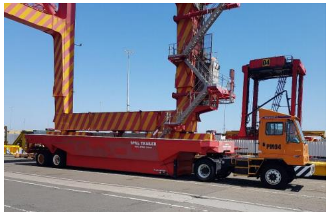
Photo 6.6.4: Spill trailer connected ITV/Mafi located mid-way on the wharf
