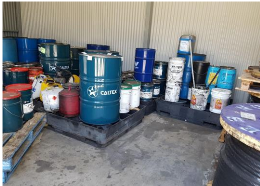
Photo 6.9.1 Oil & Grease store – oils on plastic bunded pallets and grease (due to high viscosity) on wooden pallets
