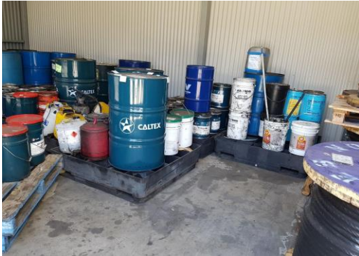
Photo 6.9.1 Oil & Grease store – oils on plastic banded pallets and grease (due to high viscosity) on wooden pallets
